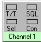
A light green band indicates that the channel is in the monitor mode and also that incoming audio is present on the channel.
