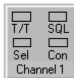
With the channel button in the greyed out state the channel is available to the operator but they have not selected it to monitor or transmit. The operator will not hear any audio present on the channel.
