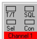
A red bar across the bottom of the channel button indicates that the operator has selected the channel and also that he is transmitting on the channel.
