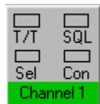
A dark green band across the bottom of the channel button indicates that the channel is selected and that incoming audio is being received on the channel.
