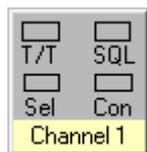
By clicking the channel button once, the channel is now available to the operator to monitor the audio present. The operator cannot transmit on this channel. A yellow band across the bottom of the button (or a solid yellow colour to the button) indicates that the channel is in the monitor mode.
